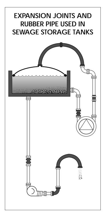
Consultants take advantage of Redflex rubber pipe and fittings to allow design flexibility. The diagram to the left, of an aeration sewage system, is one example of where Redflex products are used.
