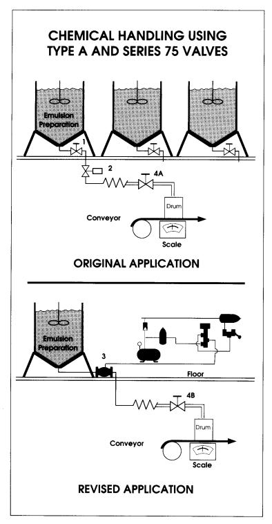
This bulk chemical company uses pneumatic Type A Valves and Series 75 Red Valve Pinch Valves due to the clumping and clogging nature of its chemical emulsions in this low pressure shear sensitive emulsion production process. This system, with 48 production tanks, previously used diaphragm valves exclusively. Space efficiency is necessary due to the method of tank installation in close proximity to the floor. Very little room was available to get to valve number 1 for emergency operation.
