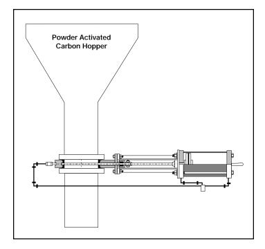
A plant in Oklahoma that manufactures Chemical Carbon Black was unable to find a valve that would work for their application. The carbon black was stored in large hoppers, and discharged by gravity through an isolation valve. The material is in powder form, and kept at 250°F. This hot, abrasive material would quickly score plug and ball valves, causing them to leak. Other styles of knifegates were also tried, but all suffered the same problems.
