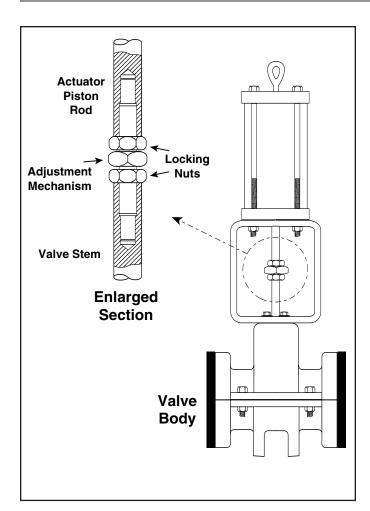
The Stroke Adjustment Unit is standard on all Red Valve Series 5200 Control Pinch Valves. The unit consists of a three-piece assembly which fits between the actuator's piston rod and valve stem; this allows the user easy field stroke adjustment of up to 1" on the Series 5200 Control Pinch Valve sleeve.
