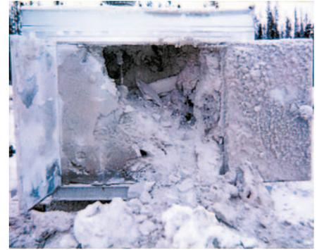
*Catastrophic failures with V-Ball valves would fill the skids with sand.*
