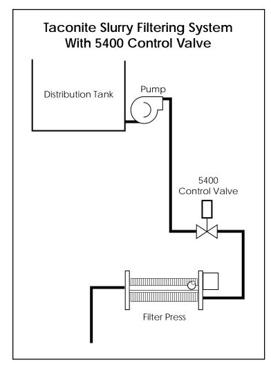
Series 5400 Control Valves are being used to regulate the flow of taconite slurry from a distribution tank to a Filter Press, which separates the water from the taconite sediment. Process level in the filters must be maintained to prevent overburdening the Filter Press. Water in the Press is drawn from the sediment with suction.
