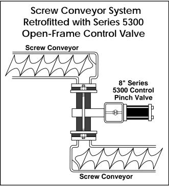
A major chemical company in the south selected Red Valve's Series 5300 Open Frame Control Valve to replace the alloy 20 butterfly valve and the expansion joint that was used to control the flow of fluorspar between the two screw conveyors. The butterfly valves would not provide a tight shut off when needed causing a backflow of the hydrofluoric gas.
