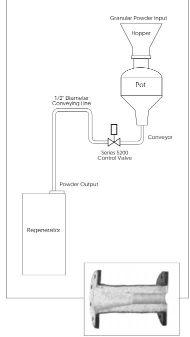
This application is for a control value to pass 80 mesh granular powder material at  $50#/ft^2$  density, with 25 standard cubic feet per minute of conveying air at about 60-100 psig.
