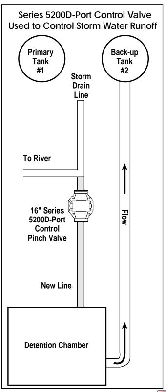
A pulp and paper mill was faced with a mandate from the EPA. They must be able to divert their storm water in case of an emergency overflow from their solids handling tanks at the Saw Mill Operation area of the plant. Their storm water runoff presently discharges straight to the river.
