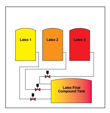
A chemical maufacturer needed to mix 3 different latex fluids into one compound that would eventually be used as a backing for carpeting. It was important to maintain the correct ratio of the three compounds, so precice a control valve was needed.
