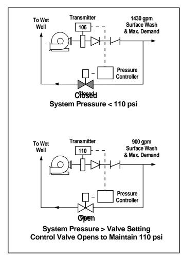
Red Valve's Series 5200D-Port Control Pinch Valve was specified for this Texas Washwater Pumping station. The valve is used to maintain a constant pressure in the pump discharge.
