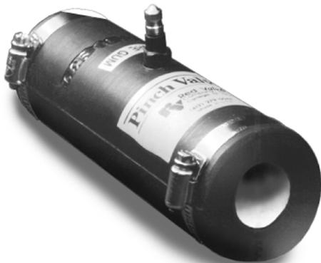
Red Valve's Type R All-Rubber Pinch Valve is an ideal valve for water, chemicals, solids and slurry applications. The valve is easily installed between two pieces of pipe with hose clamps. Simply add 20-psi air pressure over line pressure and the valve closes drop-tight. For example: If process line pressure is 45 psi, 65 psi closes the valve. It's that simple!
