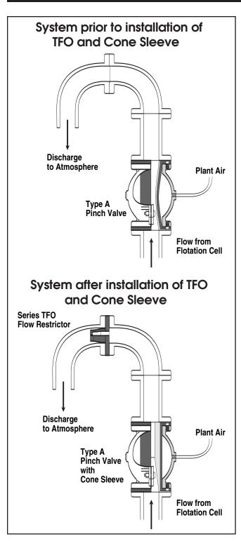
While visiting the world's largest copper mine, Codelco's Chuauicamata Mine, Red Valve's products were widely seen. The most common valves were the Type A Pinch Valve on throttling service. Since the installation of these valves, numerous problems have been solved using Red Valve's patented Cone Sleeve and TFO.
