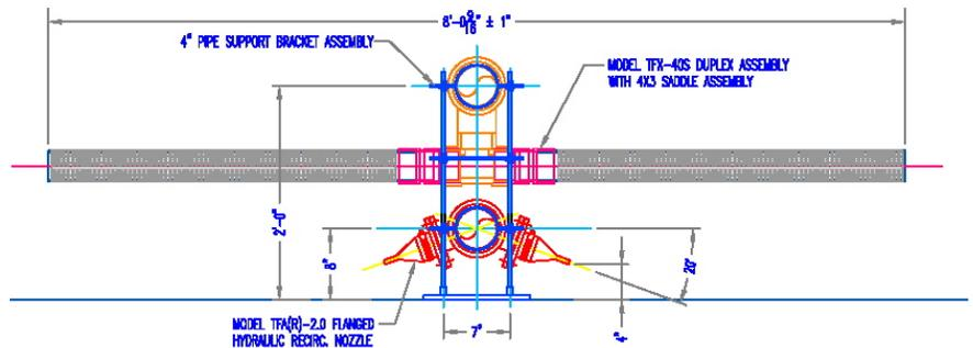
Re-suspension of settled solids after decanting periods is critical to the performance and efficiency of the SBR process. The Tideflex hydraulic
