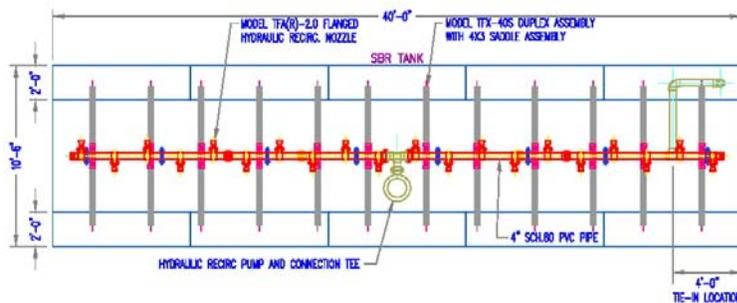
mixing nozzles are oriented toward the bottom of the tank and produce a duplex roll pattern, this provides immediate re-suspension of the settled biomass. During the aerobic cycle the hydraulic mixing system can be operated continuously or periodically to maintain solids suspension; the fine bubbles discharged from the tube diffusers are retained longer within these mixing loops increasing their transfer efficiency and increasing the treatment process performance.
