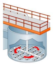
The Tideflex High Pressure Elastomeric Nozzles are constructed to withstand the forces generated by a high pressure discharge nozzle within a fluid solution. The nozzle acts as a reverse flow
