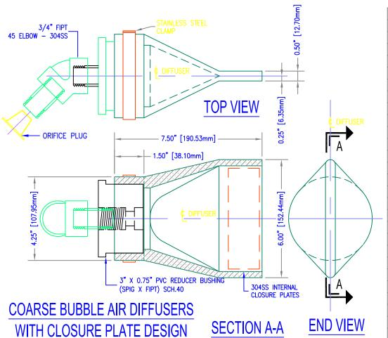
30 CFM MAXIMUM OPERATING AIRFLOW 12.5 IN. H20 DIFFUSER HEADLOSS AT MAX AIRFLOW 14.0 IN. H20 ORIFICE HEADLOSS AT MAX AIRFLOW 26.5 IN. H20 TOTAL HEADLOSS AT MAX FLOW MOLDED DIFFUSER CONSTRUCTION 304SS INTERNAL CLOSURE PLATES **EPDM** ELASTOMER MATERIAL HOSE CLAMP CLAMP TYPE 304SS CLAMP MATERIAL 304SS DIFFUSER NPT CONNECTION MATERIAL DIFFUSER NPT CONNECTION DIAMETER 0.75 ORIFICE MATERIAL 304SS NIPPLE ORIFICE TYPE 0.750 ORIFICE DIAMETER
