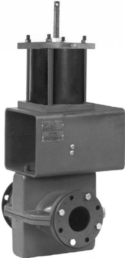
The Red Valve Series RSR Pressure Relief Valve is a bi-directional valve designed for tough slurry applications. The elastomer sleeve closes on entrapped solids in the line. The flexing action of the sleeve breaks up any sediment or build-up in the valve, which makes the Series RSR a reliable, low-maintenance pressure relief valve. A variety of elastomers are available to suit yourspecific needs.
