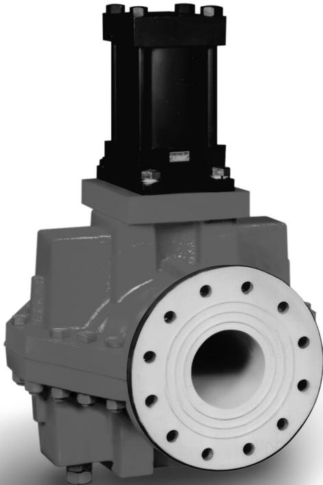
The Red Valve Series 9000 Pneumatically-Actuated Pinch Valve is a bi-directional valve designed for tough slurry applications. The elastomer sleeve closes on entrapped solids in the line. The flexing action of the sleeve breaks up any sediment or build-up in the valve, which makes the Series 9000 a reliable, low maintenance valve.
