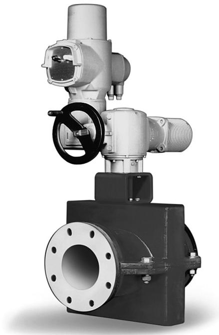
The Red Valve Series 9000E Electrically-Actuated Pinch Valve is a bi-directional valve designed for tough slurry applications. The elastomer sleeve closes on entrapped solids in the line. The flexing action of the sleeve breaks up any sediment or build-up in the valve, which makes the Series 9000E a reliable, low-maintenance valve.
