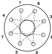
If greater torque is required, continue re-torquing in increments of 50% of tabulated values.
