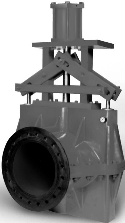
The Red Valve Series 5400 Control Pinch Valve is a bi-directional valve designed for tough slurry applications. The elastomer sleeve closes on centerline, creating a smooth venturi which reduces wear. The flexing action of the sleeve breaks up any sediment or build-up in the valve, which makes the Series 5400 a reliable, low maintenance control valve.
