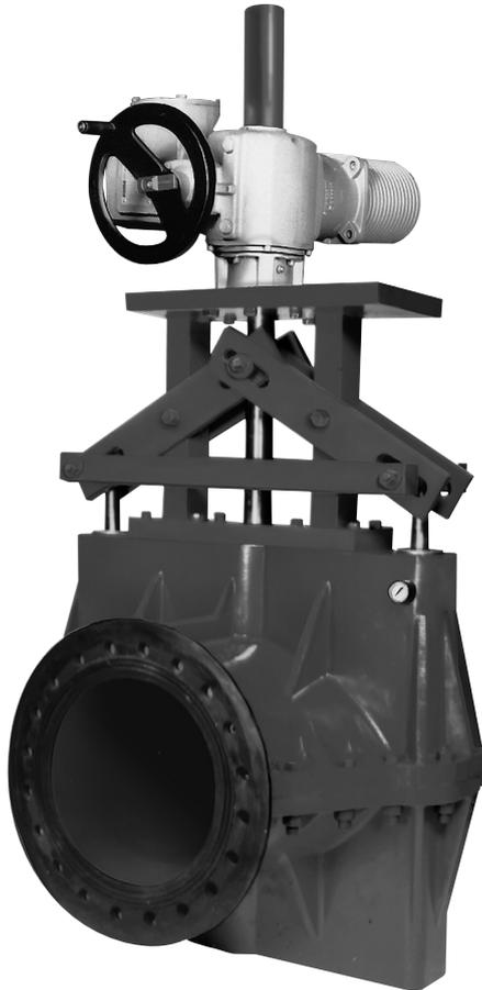
The Red Valve Series 5400 Control Pinch Valve is a bi-directional valve designed for tough slurry applications. The elastomer sleeve closes on centerline, creating a smooth venturi which reduces wear. The flexing action of the sleeve breaks up any sediment or build-up in the valve, which makes the Series 5400 a reliable, low maintenance control valve.
