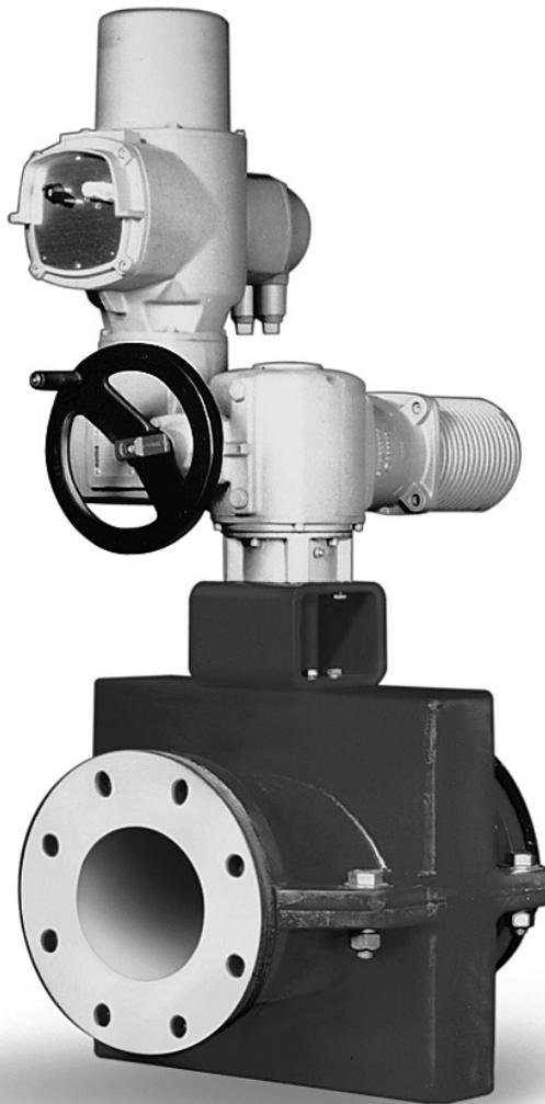
The Red Valve Series 5200E Electrically Actuated Control Pinch Valve is a bi-directional valve designed for tough slurry applications. The elastomer sleeve closes on entrapped solids in the line. The flexing action of the sleeve breaks up any sediment or build-up in the valve, which makes the Series 5200E a reliable, low maintenance valve.
