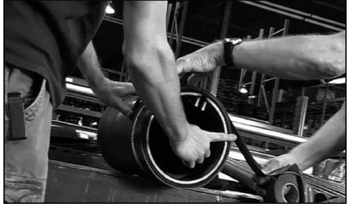
**STEP B:** Slowly rotate the valve while firmly pressing the rubber adhesive strip onto itself in concentric layers until valve O.D. is equal to or a fraction smaller than pipe I.D.
