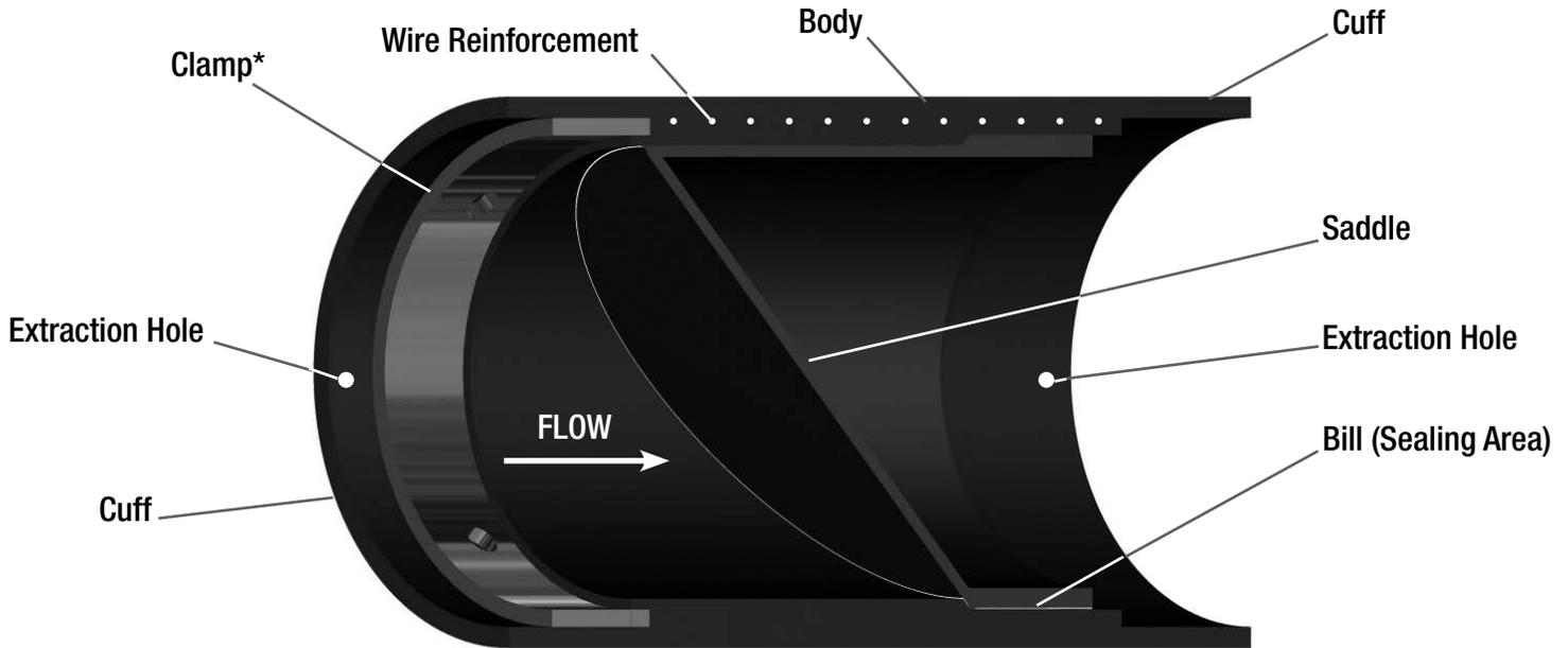
\*Clamps are installed in the upstream or downstream cuff, depending upon the application. The illustration above is shown clamped upstream.
