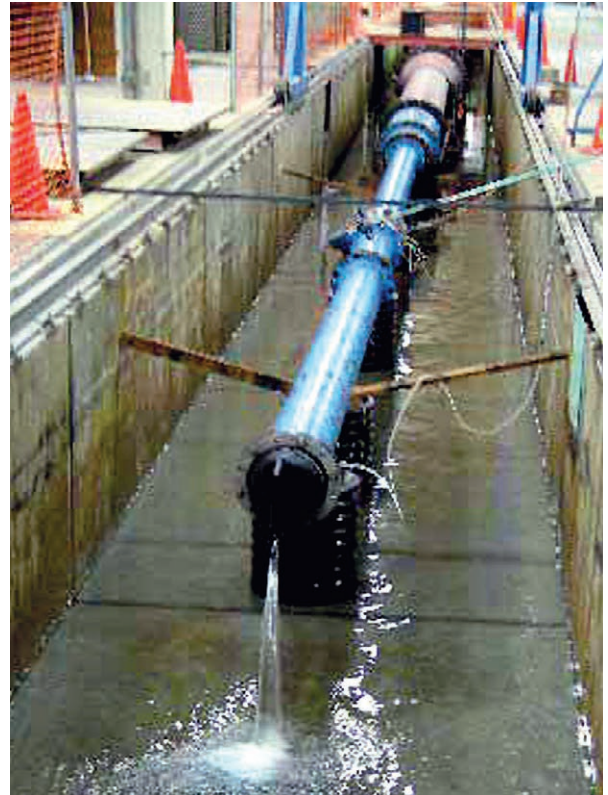
A Tideflex® Check Valve being hydraulically tested by an independent laboratory.
