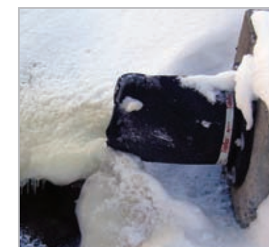
Tideflex® Valve still discharging water at -35° F.
