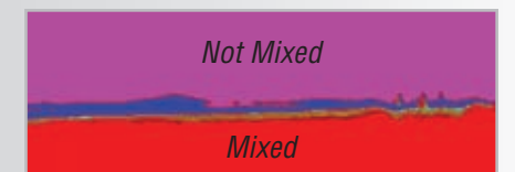
Stratified tank due to single inlet pipe.
