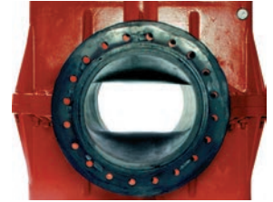
This is accomplished by the use of two pinch bars closing on centerline.
