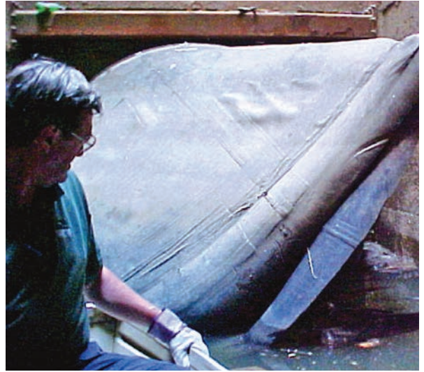
Rotating a check valve, as commonly suggested by some manufacturers, will result in distortion, gapping and leakage.
