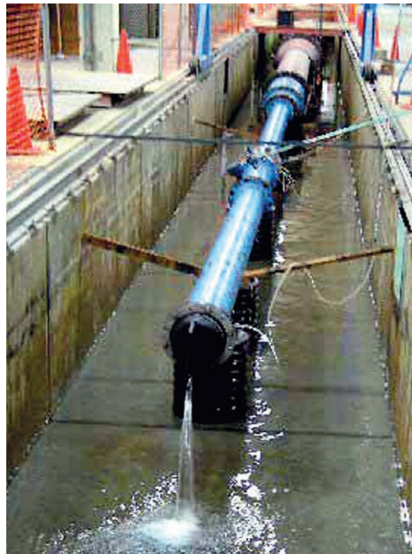
A Tideflex® Check Valve being hydraulically tested by an independent laboratory.
