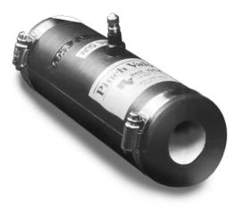
The Red Valve Type R Air Operated Pinch Valve is 100% full ported bidirectional valve designed for tough slurry applications. The elastomer sleeve closes on entrapped solids in the line. The flexing action of the sleeve breaks any sediment or build-up in the valve, which makes the Type R rellable low maintence value
