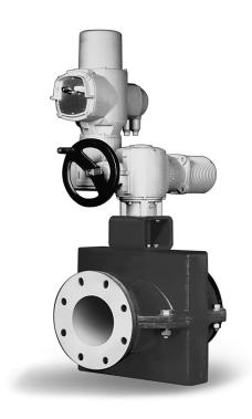
The Red Valve Series 9000E Electrically-Actuated Pinch Valve is a bi-directional valve designed for tough slurry applications. The elastomer sleeve closes on entrapped solids in the line. The flexing action of the sleeve breaks up any sediment or build-up in the valve, which makes the Series 9000E a reliable, low-maintenance valve.
