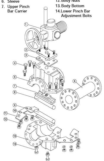
lower pinch bar can be raised by turning the adjusting nuts on the top of the guide rails clockwise. First, loosen the jam nuts, then turn the lower adjusting nut on each side rail one to two turns in the clockwise (tightening) direction. Be sure to turn each nut an equal amount. Check for complete closure of the valve. If necessary, repeat these steps until the valve seals completely. Finally, tighten the jam nuts, being careful not to disturb the setting of the adjusting nuts.
