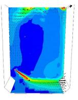
decays at a rate which is inversely proportionate to the distance it travels. A discharge plume with an initial discharge velocity of 30 ft/sec will decay to a velocity of 1 ft/sec after a 30 foot distance. Therefore, applying a single (or limited quantity) port system can result in inadequate mixing across the entire liquid volume. Multi-Port distribution systems are more able to maintain the required mixing velocities across the entire area of the process vessel.
