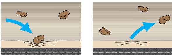
When abrasive particles strike the elastomer surface of a Red Valve Pinch Valve Sleeve, the impact is absorbed, then deflected back into the particle. These extremely resilient elastomers wear at a far slower rate than ceramic or metal alloy valve trims. Pinch Valve Sleeves are full-port with no crevices, packing glands or seats to foul valve operation.
