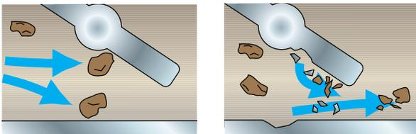
When abrasive particles strike the hard surface of traditional metal valves, the energy of the impact is completely absorbed by the metal surface, prematurely wearing seats, weirs, rotating discs, plugs and balls. Additionally, these abrasive particles can pack into crevices, scoring the sealing surface and creating leaks.
