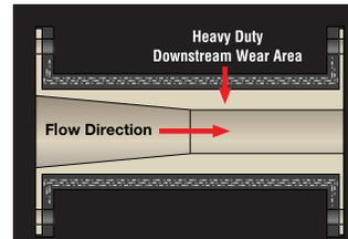
Pressure recovery occurs downstream of the sleeve, so Cone Sleeves can handle a higher pressure drop than other sleeve designs. For the same open area, the configuration of a Cone Sleeve also allows
