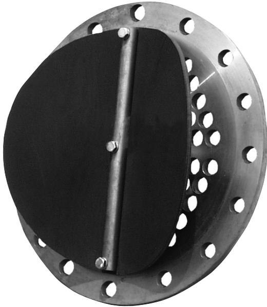
The revolutionary design of the Series WF-3 InLine Check Valve provides reliable backflow prevention. The valve solely operates on differential pressure and has no moving mechanical parts. The valve exhibits low headloss, high backpressure ratings and a short face-to-face dimension. The valve is only intended for clean flow media or media with only fine particulates. The Series WF-3 is constructed with ANSI, DIN, BS or special flange drillings for easy installation.
