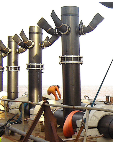
Tideflex® Diffusers discharge at an inclined angle to maximize dilution for dense jet brine outfalls from desalination plants
