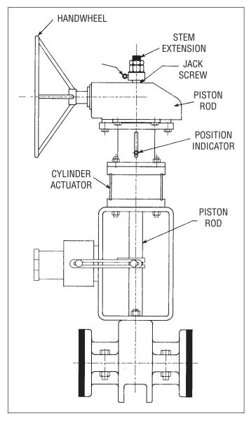
The Manual Override assembly consists of a handwheel or bevel gear actuator, a modified pneumatic actuator with a stem extension, an override mounting yoke, a position indicator and a removable override engagement pin.
