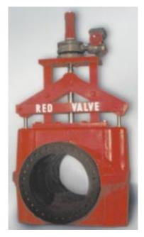
The 36" Series 5400E Control Pinch Valve is becoming quite popular as an influent flow control valve, replacing the traditional butterfly or gate valves that suffer clogging and reliability problems.
